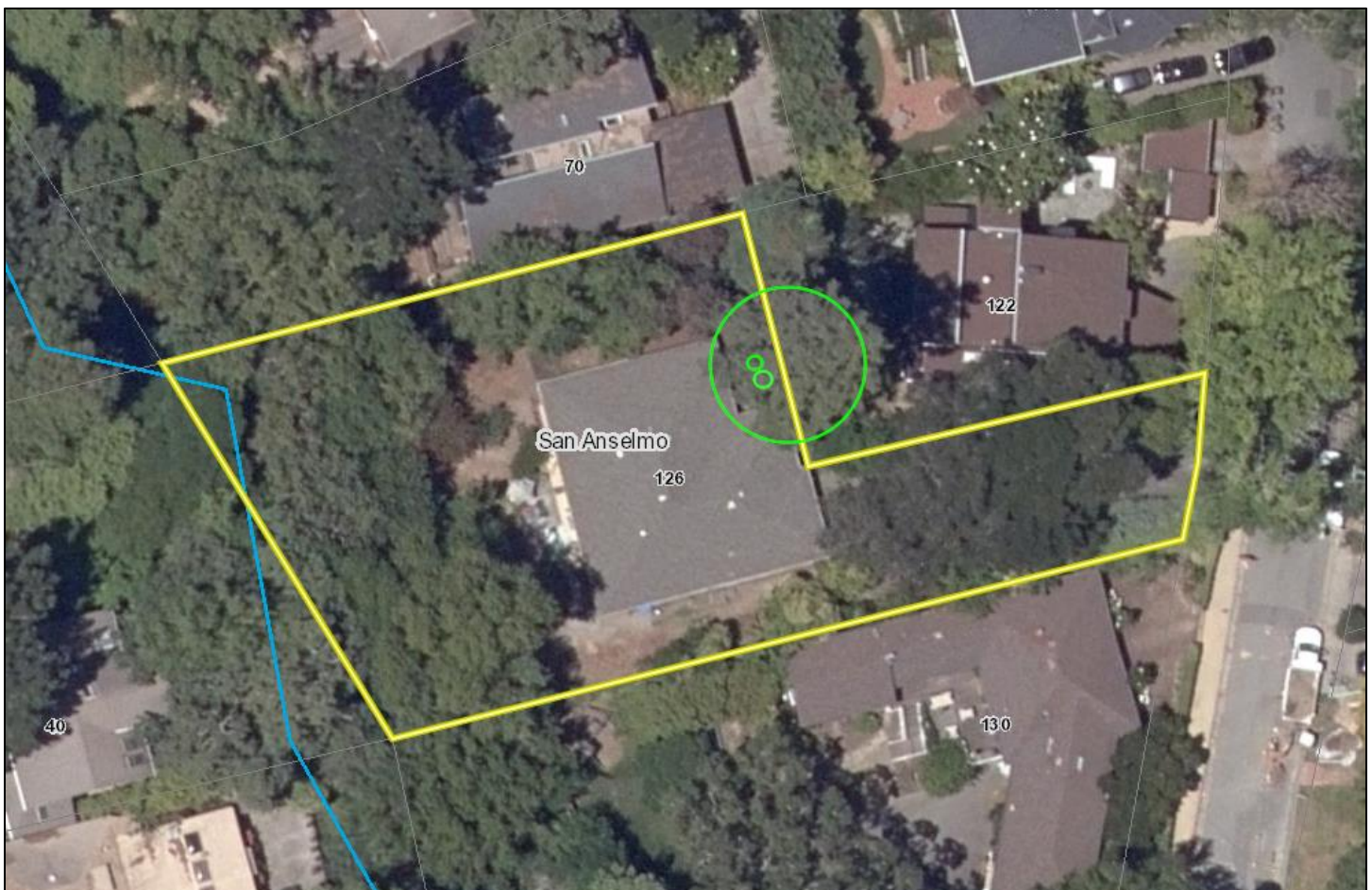
Site Plan indicating the approximate trunk locations and canopy dripline. *Not drawn to scale.
